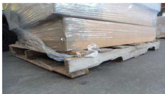
Example: Pallet without IPPC mark and poor condition
