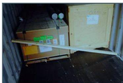
Example: Raw Wood used to lock the cargo without IPPC marks
