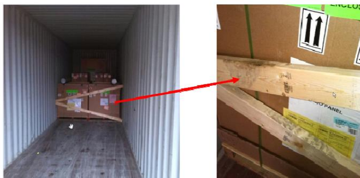
Example: Raw Wood used to lock the cargo without IPPC marks
